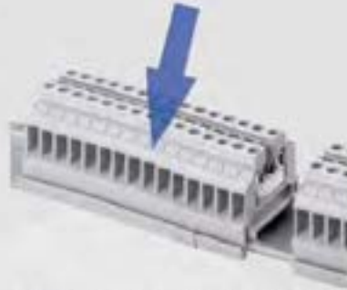
2. Snap fitting of pre-assembled terminal blocks Important: Once the terminals are mounted onto the rail, the snap-fit terminal feet are relieved from stress preventing the plastics from material fatigue.
