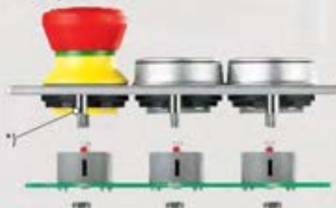
base-plate mounting using a spacer ring SDR/SDRSW mounting depth 9.2 mm
